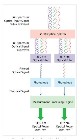
$\label{prop:prop:signal} \textit{Figure 2: Selective Optical Power Meter Schematic}$
