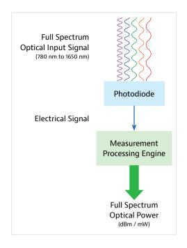
Figure 1: Broadband Optical Power Meter Schematic
