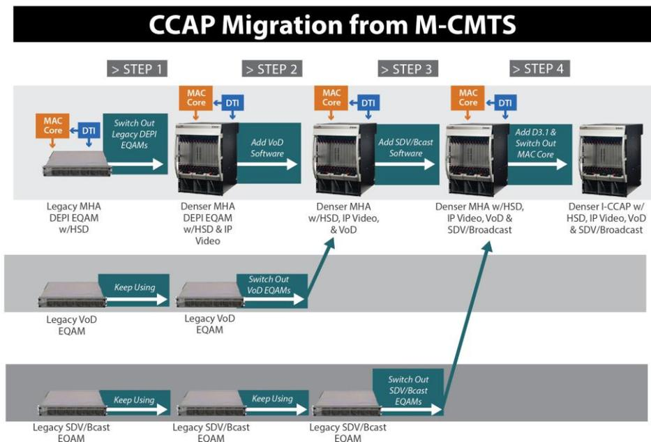
**Rationale:** This scenario applies to any service provider with modular CMTS installations. What triggers the retirement of the legacy CMTS core, or its relocation to another headend, is the need to deliver more DOCSIS channels.
