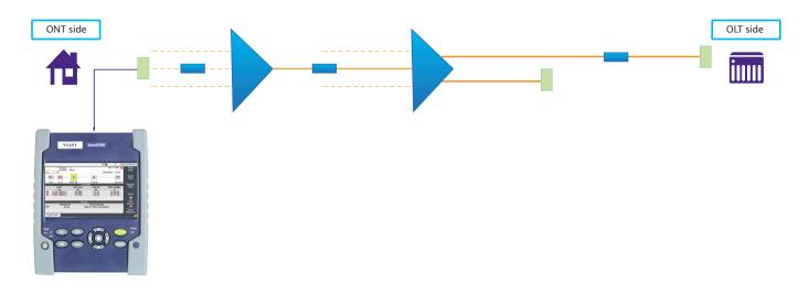
To be able to measure each segment of a PON network, testing from the ONT (customer) back to the OLT (central office), a traditional OTDR would require multiple manual tests (acquisitions) using different parameters for each. FTTH-SLM dynamically adjusts the testing parameters and automatically performs multiple acquisitions to achieve the optimum test results. All the information gathered is displayed as a single icon map view (Smart Link Mapper or SLM) and a combined OTDR trace.
