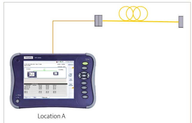
When using a single unit, FiberComplete lets users perform automatic ORL and OTDR measurements.
