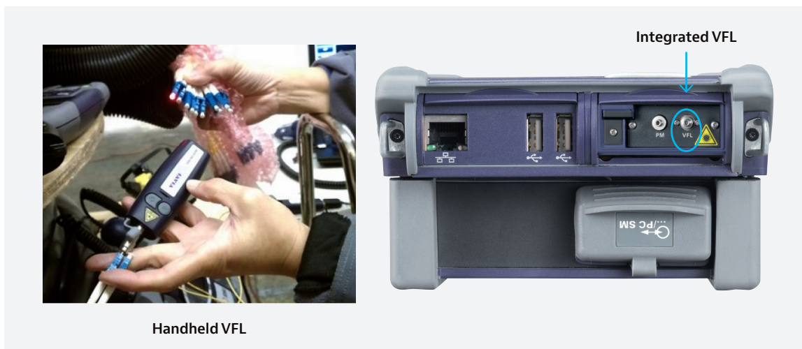
Figure 2: Fiber continuity test
