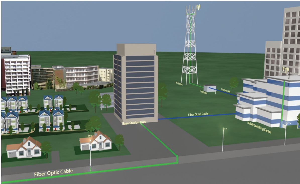
Typical FTTA radio access network layout
