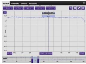
160kHz RBW -5.49dBmV 640kHz RBW 0.23 dBmV 5120kHz RBW 10.91 dBmV
