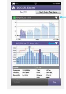
A clear picture of upstream RF performance is provided with in-channel response for DOCSIS signals
