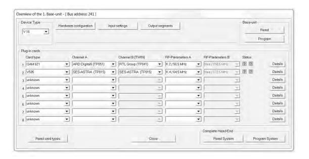
The output channels for the V 505 / X-QAM 621 card are selected under "HF parameter A" and "HF parameter B" in the planning screen of the base unit, these being the channels in which the QAM channels combined from the DVB-S(2) are fed into the cable.
