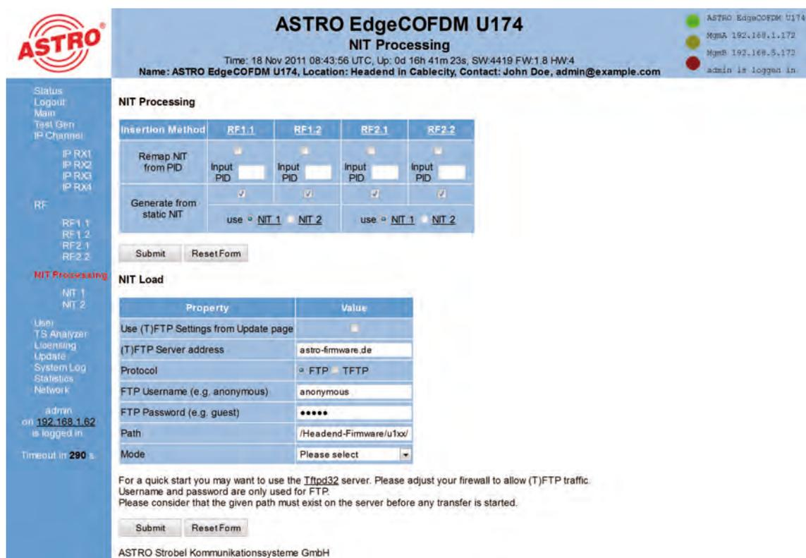
Figure 24: Activating NIT Processing / Upload NIT
