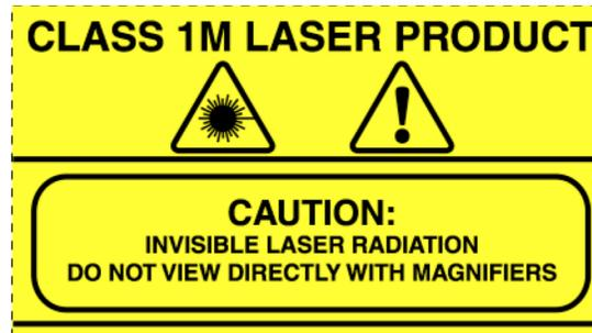
This light emission device is classified to IEC 60825-1:1993 + A1 + A2.
