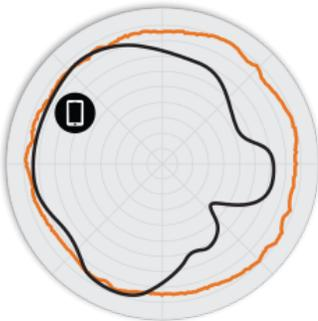
Figure 3. R320 5GHz Azimuth Antenna Patterns
