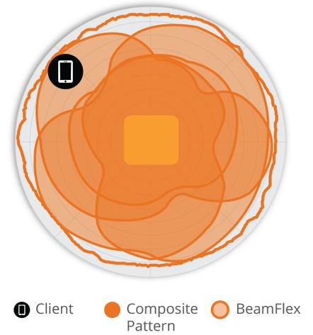
Figure 2. R320 2.4GHz Azimuth Antenna Patterns
