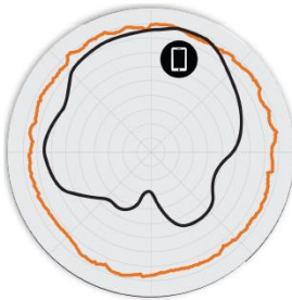
Figure 2. R850 2.4GHz Azimuth Antenna Patterns
