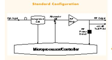
Each unit is defined during installation to have either a primary or backup personality. A primary receiver module will control both a backup module and an RF switch. If the RF output level of the primary receiver drops below the set threshold, the RF path is automatically switched to the backup receiver via the RF switch. When the primary route is restored, the path will switch back. The RF path can also be forced to either primary or backup via the HLP 4000/4200 or the NETWatch system.
