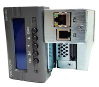
With the provided software license the HNC 4801 becomes web based SNMP proxy agent that enables users to remotely configure and control the HLP 4801 application modules. The HNC 4801 can detect alarms and send this information to a higher level network management station.
