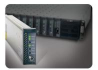
CORWave 1 GHz multiwavelength forward transmitters are an integral part of the CORWave multiwavelength plan, which operators can follow in the 1291nm region to multiplex 4 analog forward, 4 reverse, and 4 GbE-based data services wavelengths over as little as one fiber. The plan supports fiber distances of up to 30 km, forward and return nodesegmentation, and dedicated business service links in in an operator's existing HFC plant.
