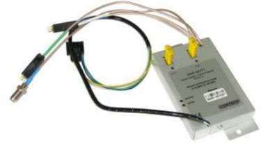
The NMT-MBxxx is a complete transponder solution for the MiniBridger amplifier from Motorola (MB89/100). Through a management SW such parameters as peak value of remote powering, operation temperature or AGC status (Automatic Gain Control) can be monitored. Furthermore the integrated return path switch enables operators to switch off or attenuate return path by 6 dB.
