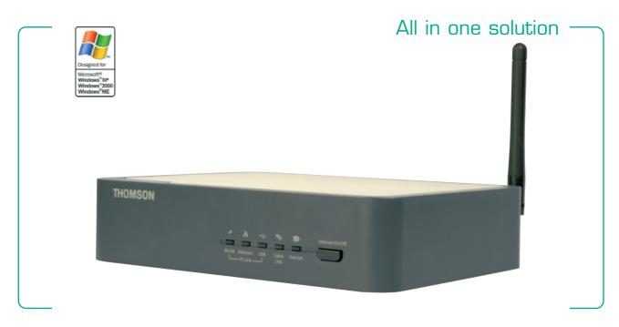
Thomson is expanding its wireless cable modem product range by introducing a Euro-DOCSIS™ 2.0 ready version, the TCW710. This gateway features an 802.11g (802.11b compatible) wireless connection with an excellent broadcast range thanks to the use of an external antenna. With the addition of CableHome™ 1.1, advanced firewall, router, one Ethernet connection and optional local
