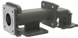
Swedish Microwave's OMT is used to separate two orthogonal linearly polarized signals simultaneously. The OMT can also support circular polarizations with a depolarizer. Greater than 31.5 dB isolation between the two linear polarizations is achieved.
